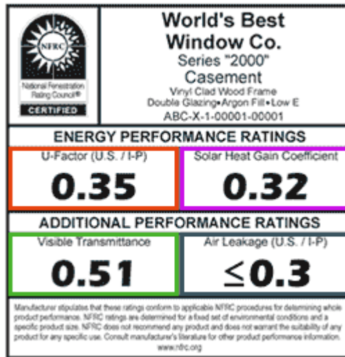
Figure 1: A sample NFRC label depicting the 3 mandatory test parameters i.e. U value, SHGC and VLT; air leakage and CR are voluntary test parameters
