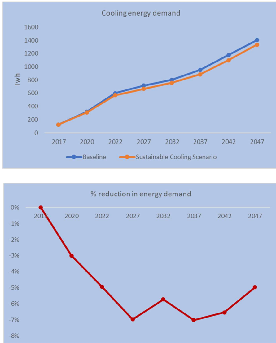
Figure 44: Comparison of cooling energy demand between BAU & STS:26C
