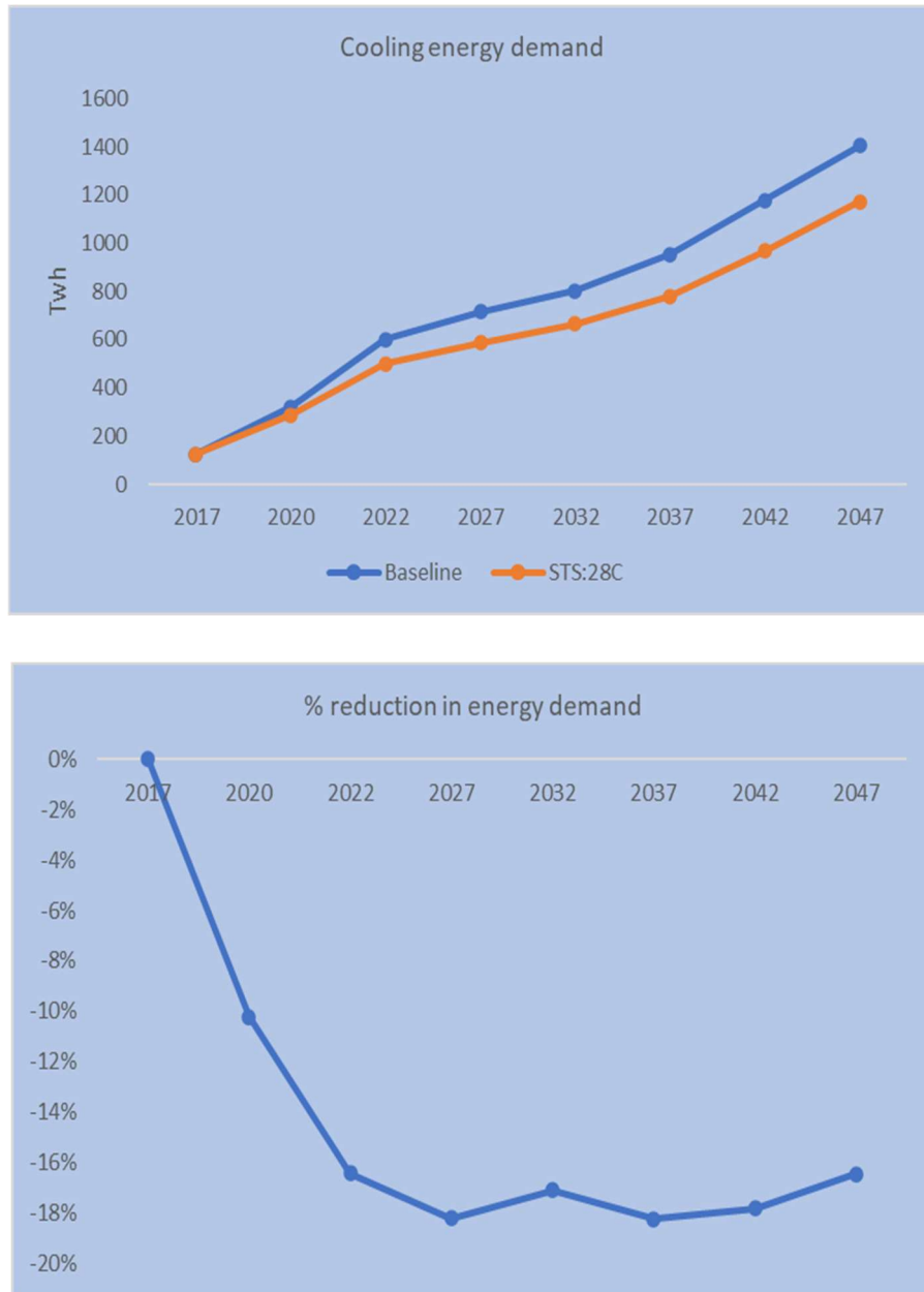
Figure 51: Comparison of cooling energy demand between BAU & STS:28C
